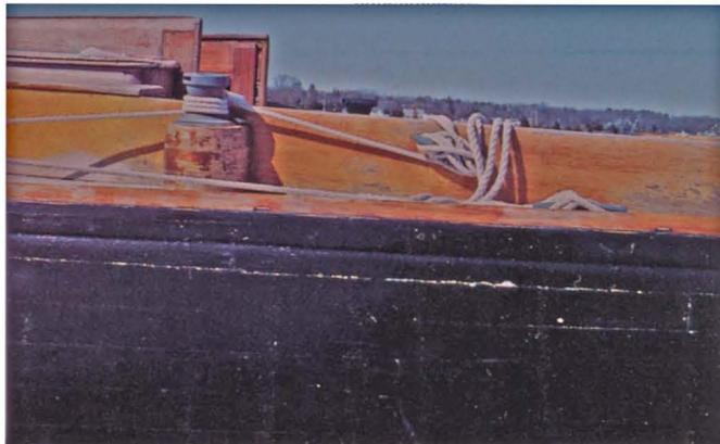
**6. The genius of Nathanael Herreshoff is obvious in this photograph.** The gorgeous sheer of the boat is set off by the care her owner has taken to keep maintenance to a minimum. Note how each seam and plank butt is visible for inspection and repair and how the toe rail drains have been kept free of debris. The bronze fittings have been allowed to weather naturally and have not been worn dangerously thin by excessive polishing.
