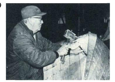
A caulking iron and wooden mallet are used to drive the cotton caulking into the hull seams. Notice that the hull's starboard side has been smoothed, but the port side is still being planked. The garboards are fastened to both floors and frames.
