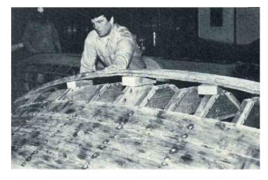
The old keel serves not only as reference for the shape and bevel of the new one, but also is used by Steve as a bending form, though it is blocked off the boat in the middle to give the new keel a slight overbend, which is always desirable. The hull, of course, has been turned over first as shown on the preceding page and blocked up so it is free from twist.
