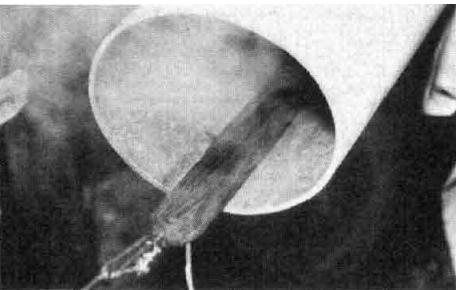
New frames of straight-grained oak are gotten out, measuring close to the right length (with an allowance of an extra 6") and having the correct heel bevel. Each is tagged for location before being put in the steambox. After steaming for a half-hour or so, the frames are taken out of the steambox one at a time and quickly handed up into the boat.
