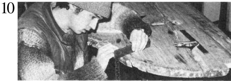
Bevels are now picked up very carefully from the old transom at each of the marked stations. This can be done in a number of ways; the method Dexter Cooper is using here involves marking the difference between the inner and outer transom faces on a piece of masking tape stuck onto a small framing square.
