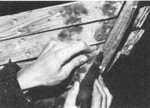
The use of thickened epoxy shows clearly in this photo. It gives the planking a new lease on life and allows these full-length cedar planks, even though slightly damaged and worn, to be used again. For a good fit the second time around, some of the plank ends are dressed down with a block plane, as shown.
