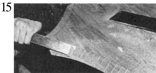
With a slick, a chisel, and later with a spokeshave and block plane, the wood between the saw cuts is removed and the beveled edge trued up.
