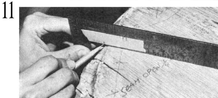
This is the time to correct any gaps that existed between the transom and hull planking before the old transom was taken out. While the upper part of this transom appeared to fit well enough, it will be necessary to close up the gap or seam starting at station 7, as noted in pencil on the old transom before its removal.
