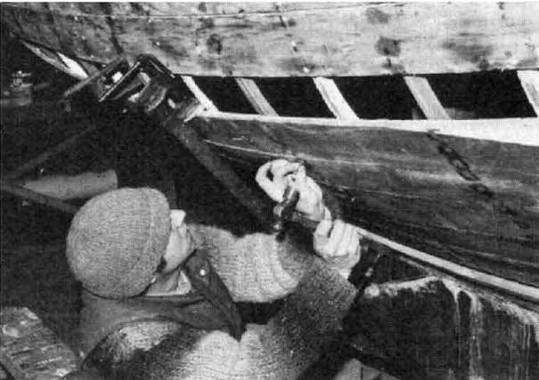
Copper rivets are then driven through each of the holes, most planks having three rivets per crossing. A nail set drives them all the way into their counterbores. Although it's doubtful that they'd ever leak, just to be on the safe side Dexter wraps a strand of caulking cotton around the shank of each rivet just under its head. The cotton is held there with the sticky bedding compound he daubs on beforehand.
