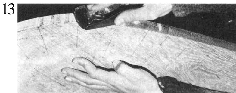
The outermost of the two lines, representing the inner face of the transom, can then be sawn out and planed square, fair, and to the line.
