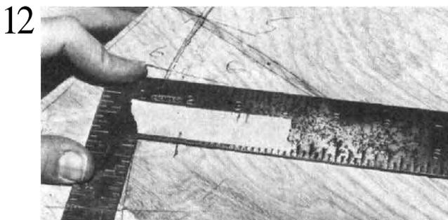
The mark on the tape is now transferred to the new transom, and after all the stations have been so marked, the marks are connected with a fair line run through them.
