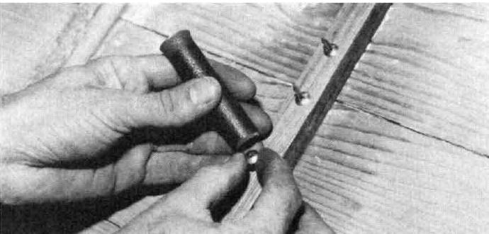
Now for the burrs, or roves, as they're sometimes called. These are a force fit over the rivet shanks, and a short length of round bar with a hole drilled along its axis serves as a tool to drive them on.
