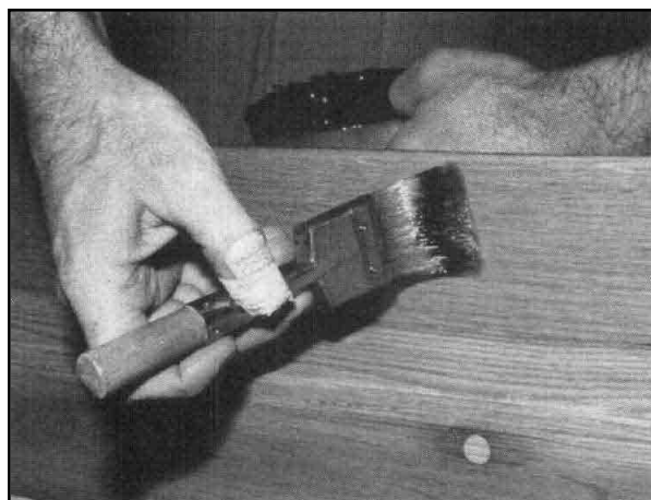
Any runs off the top edges must be picked up and blended into the coating now being applied to the sides as on this outside face, for example. Every brushful of newly laid-on varnish is brushed out until it feels and looks smooth and even. Jason is doing only the vertical side of the coaming, stopping at the covering board, which will be done separately afterwards.
