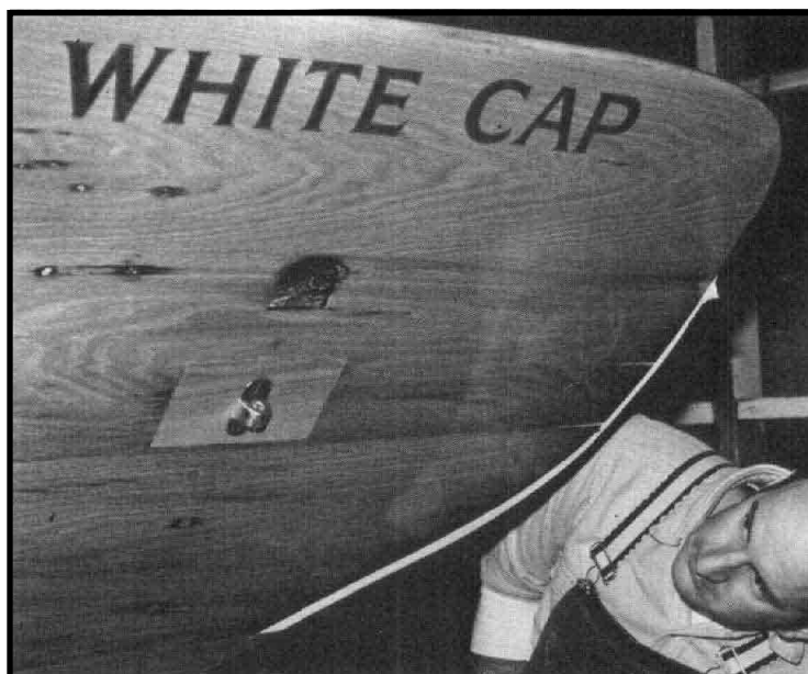
Frequent sighting for runs, sags, and bare spots while the varnish is still wet enough to make corrections is very necessary. These imperfections show up better, of course, in good light. Note the graving piece or dutchman set into the transom in way of the rudder gudgeon, and the newly painted name—applied just before the final coats.
