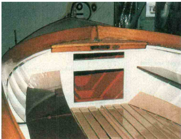
Paint on the hull interior and floorboards, and installation of the newly varnished seats just about completes the job on WHITE CAP, except for reinstallation of the hardware.
