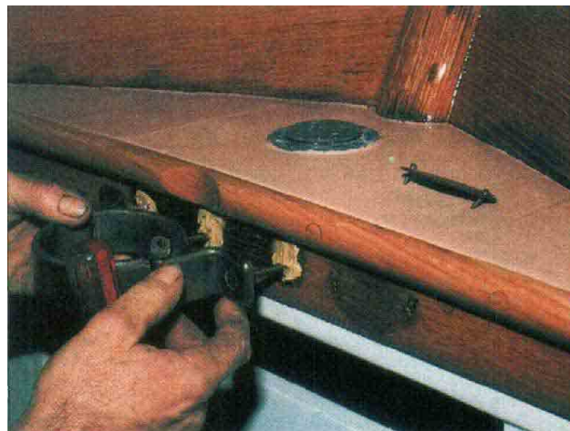
Bedding compound, along with the good buildup of varnish over the wood, will keep moisture out from behind fittings—like the mast partner bale—for a long time to come. While the metal fittings were off, they were cleaned of old paint and varnish and buffed up a bit, both jobs being made easier because the fittings weren't left on the boat. The Herreshoff nameplate lies on the deck—the next item to be put back in place.
