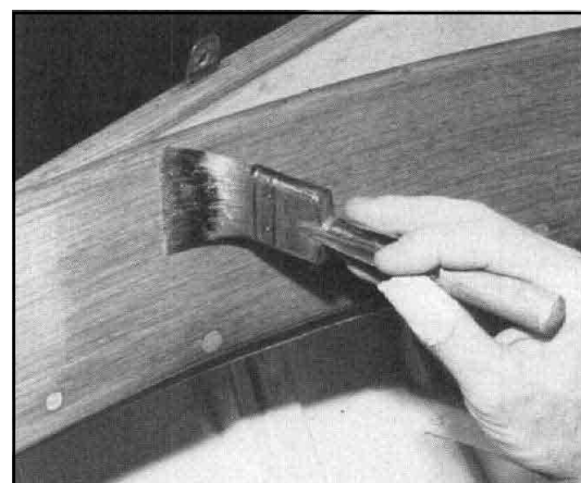
Now the same treatment is given to the inside face of the coaming, always stroking back into the already-varnished area with the final smoothing.
