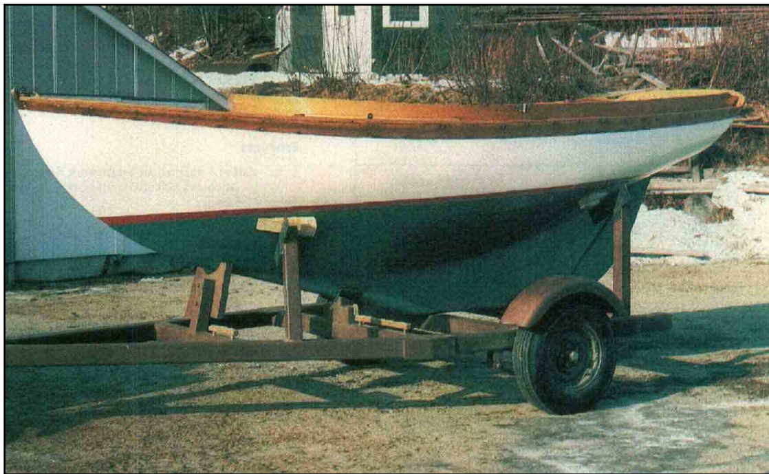
Before coming to Riverside, WHITE CAP had been reframed and repaired in a mediocre way, and there was considerable time devoted here to making her look good in spite of this history. She had somehow developed a noticeable hump in the sheerline on both sides forward. New toerails, made higher where they join the stem, and lower in the way of the hump, helped make her sheer look presentable, as did a faired-out and somewhat higher paint line at the bottom of the sheer strake forward. The new gar boards, however, which were apparently installed at the same time, aren't completely fair with the rest of the bottom planking as can be seen in the photo.
